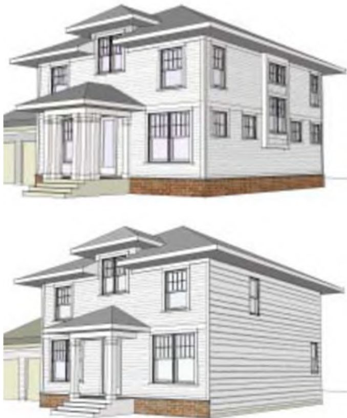
The top example shows window and trim details that are consistent on all sides, but the example below lacks such architectural features.
